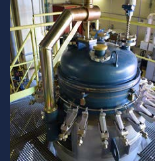
^ Our PHYre® pilot-scale process to recover carbon fibers from composite materials
